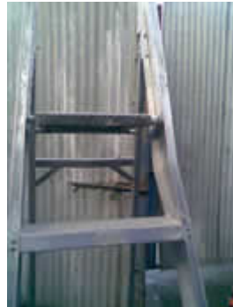
Ladder with bent support
